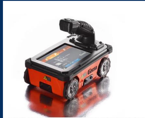
Photograph 8: AEI's in-house GSSI Mini XT scanner used during the field review.
