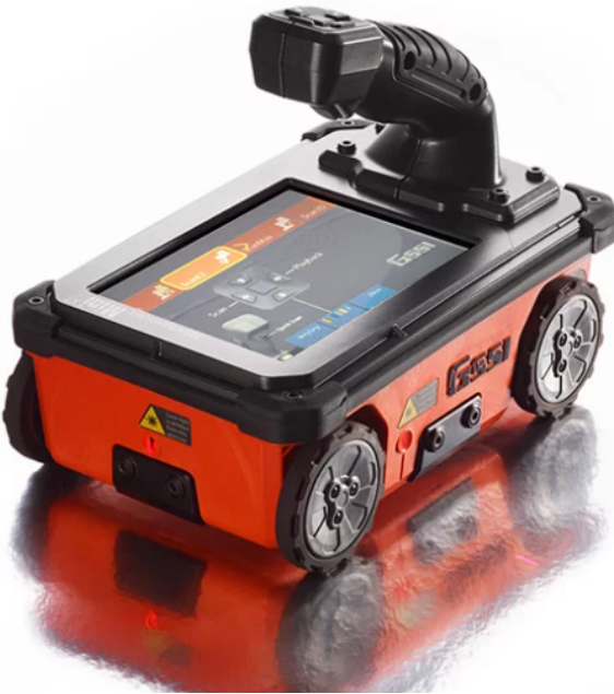
Photograph 8: AEI's in-house GSSI Mini XT scanner used during the field review.
